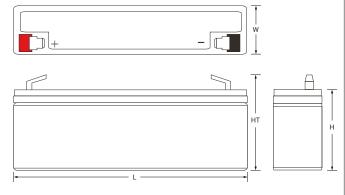
L: 7.00 (178) W: 1.37 (35) H: 2.36 (60) HT: 2.59 (66) Tolerances are +/- 0.04 in. (+/- 1mm) and +/- 0.08 in. (+/- 2mm) for height dimensions. All data subject to change without notice.
